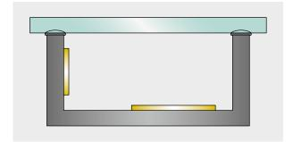
LDS structures (gold) can be placed in areas where this was not possible before, e.g. compact, closed components
