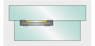
The use of LDS material (grey) can be limited to specific areas that are subsequently welded form-fittingly to the larger part
