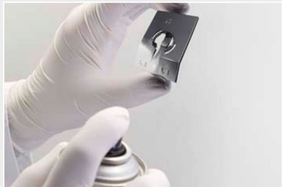
2. Painting the part with LPKF ProtoPaint LDS
