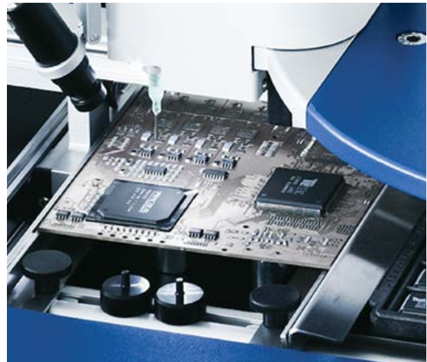
The vacuum needle places the component exactly in the desired location
