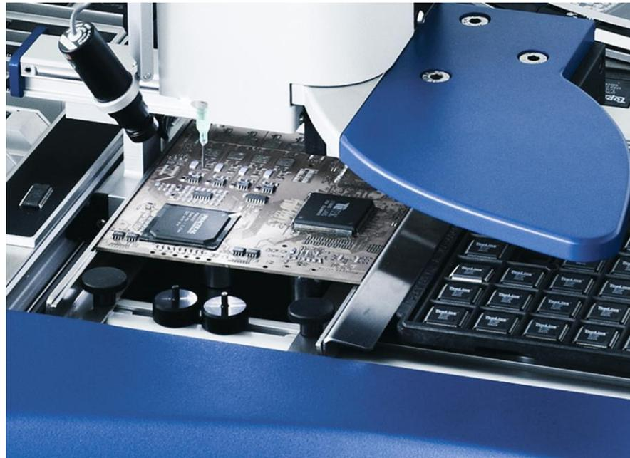
The assembly of the finished printed circuit board is carried out with the help of the **LPKF ProtoPlace S**.
