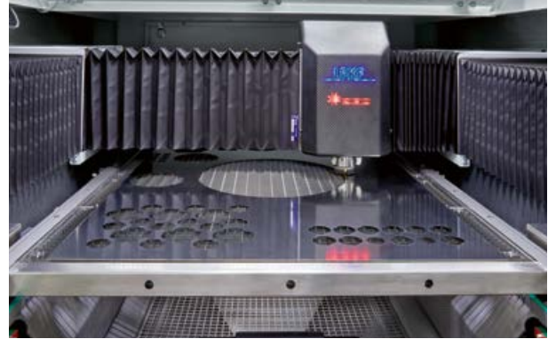
Flatbed frame used with the StencilLaser G 6080
