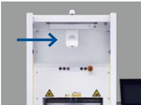
LPKF TherMoPro for the thermographic check of the weld seam
