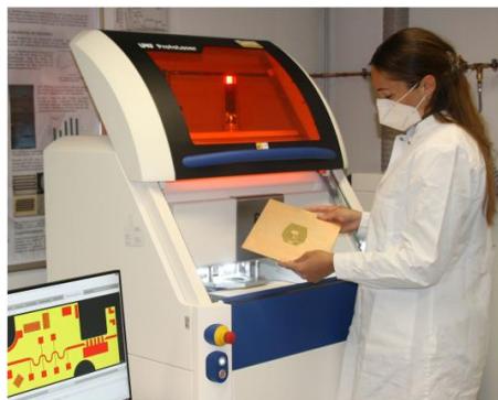
Fig. 2: Ultrafine structuring of a circuit board Photo by C. Wißler / University of Bayreuth
