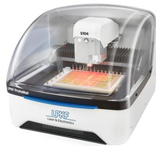
Fig. 3: The LPKF ProtoMat S104 circuit board plotter is a special system that is particularly suitable for creating applications with HF materials.
