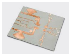
Fig. 4: Milled filter design on sensitive high-frequency material
