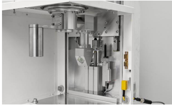
Fig.: The rotating arm in the LPKF InlineWeld 2000 enables high-precision beam guidance in the laser welding process.
