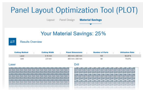
Fig. 1: Result of sample calculation of materials savings that can be achieved with laser cutting for a standard trade show sample. Although the PCBs already make optimum use of the panel space for the milling process (right), a material saving of 25% is possible for the entire panel with the laser full-section cut (left).
