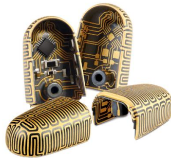
Fig. 2: Artificial fingertips: For use in prosthetic or robotic hands, conductive circuits can be precisely applied inside and outside using LDS technology. This enables improved functionalization of the fingers.
