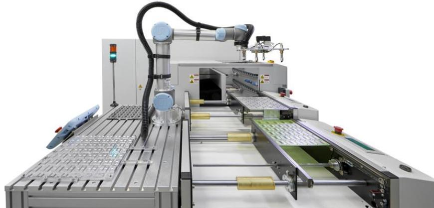
**Fig. 2:** With the help of a cobot, the panels are positioned on a specially designed tray before cutting, and subsequently collected from it. High throughput is made possible by the use of two carriers, which are operated alternately and thus allow the processing of two process steps at the same time.
