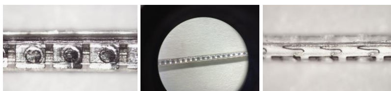
Figs. 1a, 1b, and 1c (alternative): 32-channel cochlear electrode arrays manufactured using the LPKF ProtoLaser R
