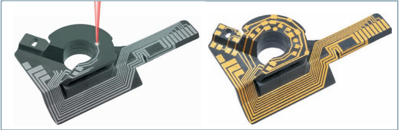
4 The layout of a structure can be adapted on the computer in little to no time and immediately transferred to the component (Image: Iskra)
