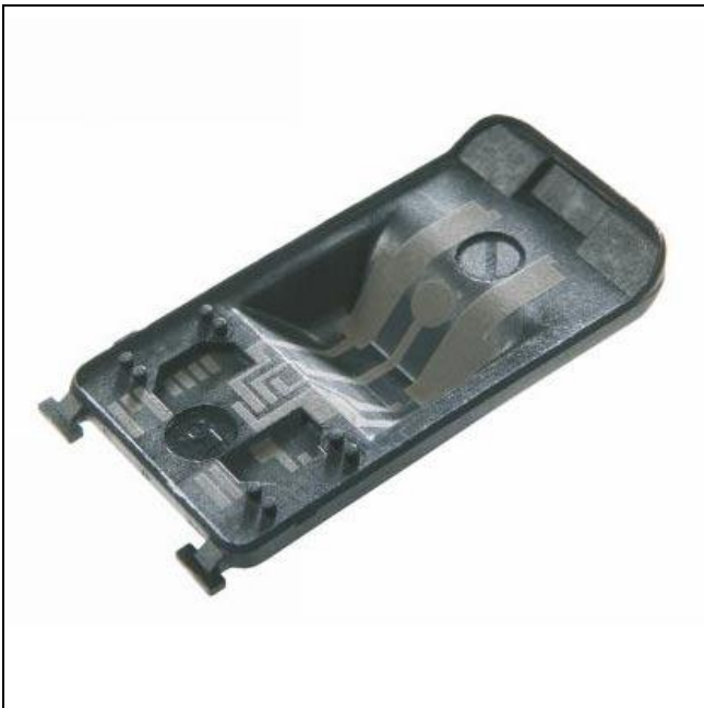
Picture 3: Plastic part after laser activation
