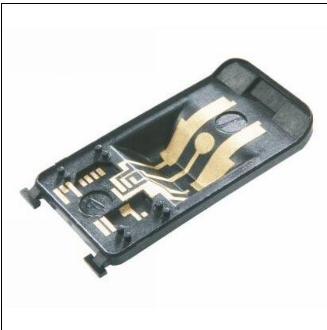
Picture 4: Plastic part after metallization
