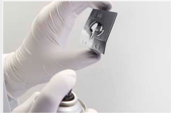
2. Painting the part with LPKF ProtoPaint LDS
