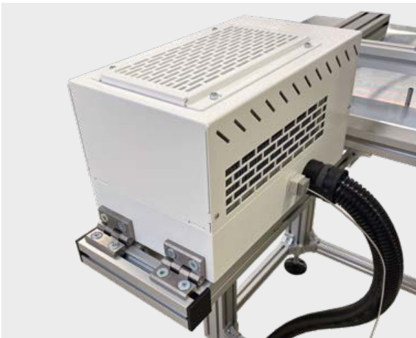
Option: external air-cooled laser box for more machine layout flexibility
